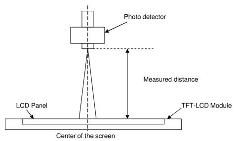
Note 2: Definition of viewing angle measured by ELDIM (EZContrast 88)
